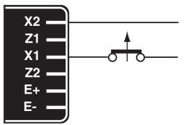
The exciter is switched off by disconnecting the AVR power supply (1 wire - X1 or X2). Contact rating 16 A - 250V A.C.
