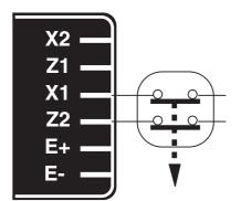
The exciter is switched off by disconnecting the AVR power supply (1 wire on each auxiliary winding) - contact rating 16 A -250V A.C. Connection is identical for resetting the AVR internal protection.
