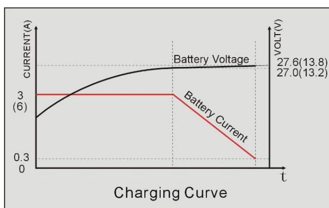
According to the characteristic of lead-acid battery, 2 stages charging method, when the battery voltage is under default value, charging for constant-current, when the battery voltage is much higher default value, the charge current is decrease following by the charge voltage increase, until it preset float voltage, then
