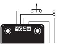
The exciter is switched off by disconnecting the AVR power supply (1 wire - 0 or 110V). Contact rating : 16A - 250V alt.
