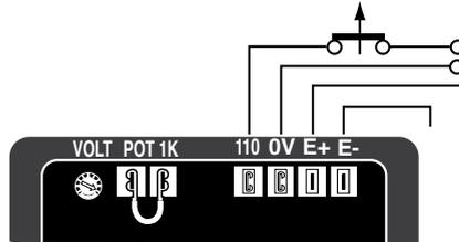
The exciter is switched off by disconnecting the AVR power supply (1 wire - 0 or 110V). Contact rating : 16A - 250V alt.
